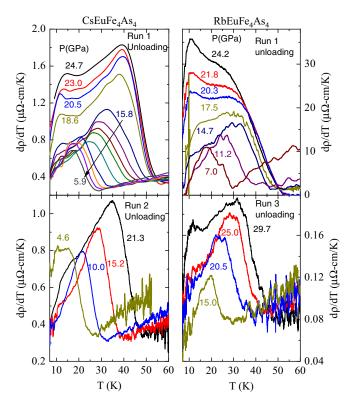
FIG. 7. Derivative of the resistivity as a function of temperature for several different pressures while unloading in the regime where  $T_m > T_c$ . Data for two different pressure runs are shown for both CsEuFe<sub>4</sub>As<sub>4</sub> (left) and RbEuFe<sub>4</sub>As<sub>4</sub> (right).
