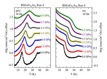
FIG. 3. Measurements of the dc susceptibility of RbEuFe<sub>4</sub>As<sub>4</sub> plotted vs temperature for several different pressures. The left and right show the zero field cooled (ZFC) and field cooled (FC) data. The data have been offset for clarity.
