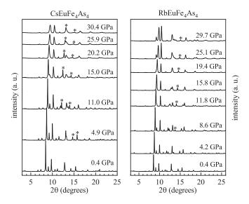
FIG. 1. Selected XRD patterns for  $CsEuFe_4As_4$  (left) and  $RbEuFe_4As_4$  (right) at various pressures. The data were taken at room temperature. Solid Ne peaks are identified by asterisks in the spectra at and above 4.9 GPa.
