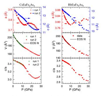
FIG. 2. Lattice parameters, unit cell volume, and c/a ratio versus pressure for CsEuFe<sub>4</sub>As<sub>4</sub> (left) and RbEuFe<sub>4</sub>As<sub>4</sub> (right).
