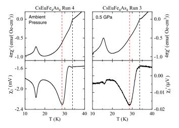
FIG. 4. Real parts of the first and third harmonic as a function of temperature for a large piece of CsEuFe<sub>4</sub>As<sub>4</sub> at ambient pressure (left) and a small piece inside the diamond anvil cell (right). The vertical dashed lines are guides to the eye showing the correspondence between features in the first and third harmonic. The minimum in  $\chi_3'$  occurs near the midpoint of the superconducting transition in  $\chi'$ .
