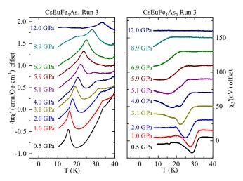
FIG. 5. The ac magnetic susceptibility as a function of temperature for CsEuFe<sub>4</sub>As<sub>4</sub>. (a) Real part of the first harmonic ( $\chi'$ ). The superconducting transition is visible as a drop in the signal and the magnetic transition corresponds to the peak. (b) Real part of the third harmonic ( $\chi'_3$ ).
